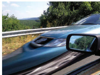
Wikipedia Example: Artifacts of rolling shutter under motion
